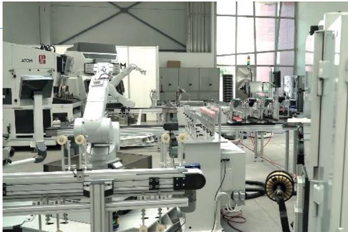
tomated line. The strong point of this solution is the great flexibility: it can be designed and scaled according to the customer's production needs, it can work all types of footwear (with very few exceptions), and it can use existing lasts without any modifica-
